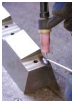
Using TIG (GTAW) to repair base material using Anviloy® Weld Rod
