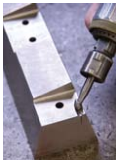
Using TIG (GTAW) to repair base material using Anviloy® Weld Rod
