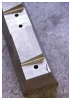
Using TIG (GTAW) to repair base material using Anviloy® Weld Rod
