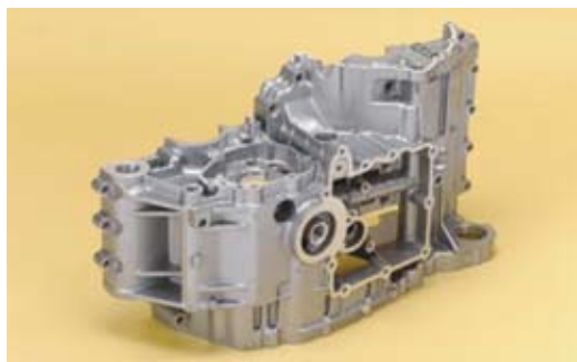
Typical casting using Anviloy® material for some die components
